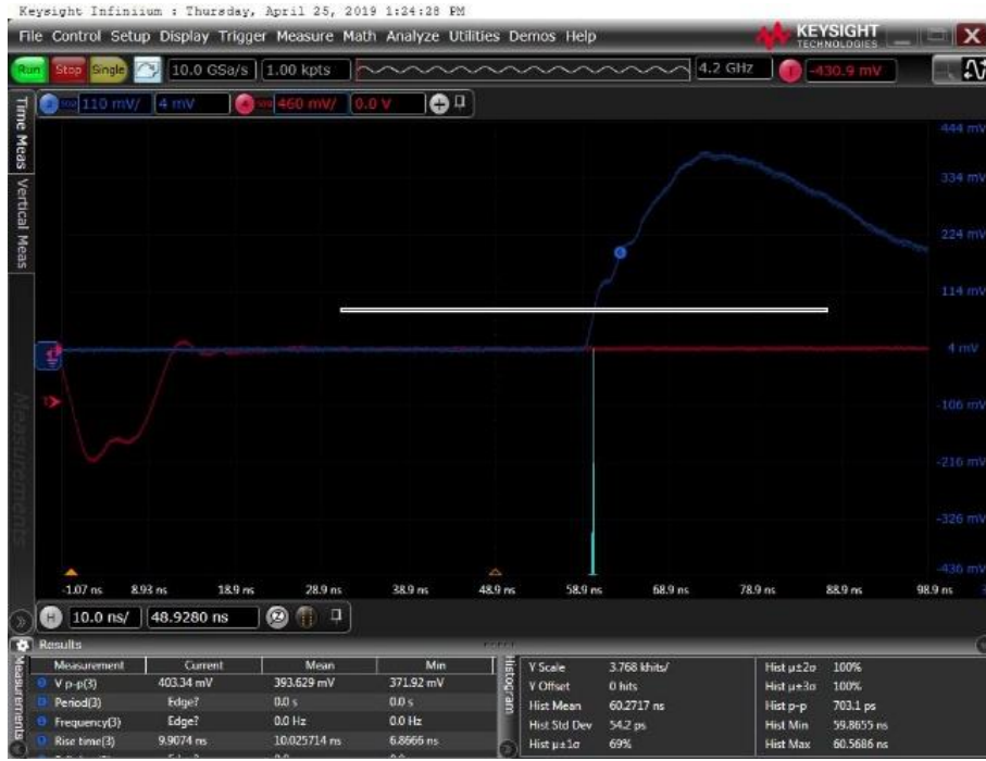
Figure 3. Image showing an example for the measurement performed using the oscilloscope (not to scale), where blue signal refers to SiPM output and red is the trigger signal. A threshold is also seen on the blue curve and the histogram (in cyan) build up below it.
